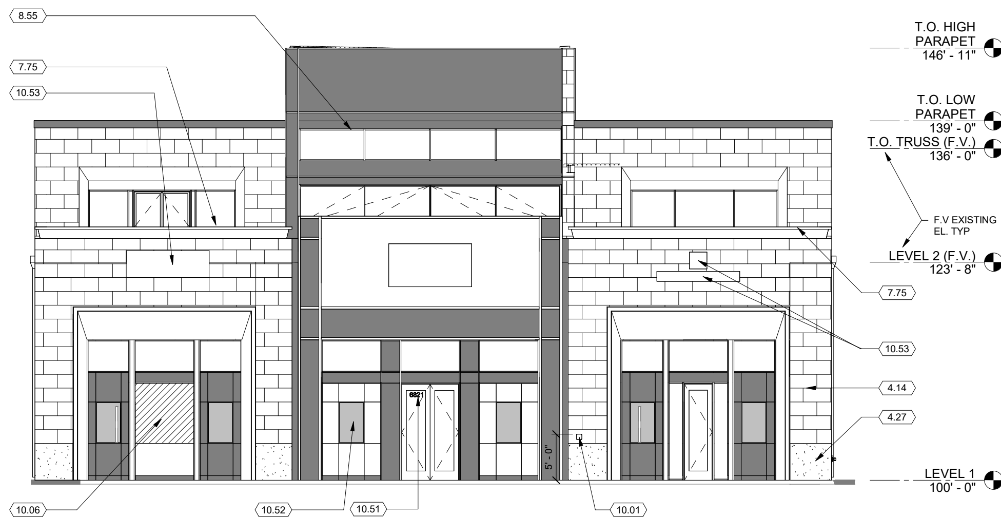
1 EAST ELEVATION REMODELED SCALE: 1/8" = 1'-0"
