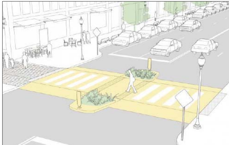
Figure 11 - Colored Raised Crosswalk
