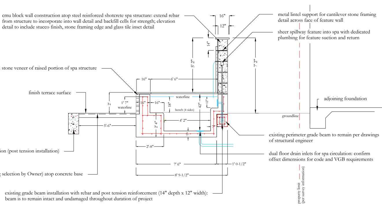
note: new steel reinforced spa structure to be placed in front of and atop existing grade beam structure with 7" wall and floor cross section detail at beam; include placement of 1/2" expansion material across top and face of beam structure
